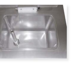
**Mixing and heating tank**. Heating occurs by means of the circulation of glycol (bain-marie) which prevents the product from burning. Effective mixing of the ingredients, directly in the tank, is carried out using a gear motor that prevents foam from forming. Precise temperature control allows 3 programs that can be
