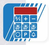
**Heating controls**, include all keys needed to turn the functions performed in the upper tank On and Off:
